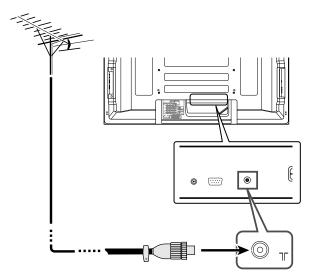
• For viewing analogue broadcasts only, connect the 75-ohm coaxial cable (commercially available) to ANT (analogue input) terminal.
